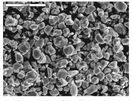
**Fig.4.** The morphology of jet-milled powder pulverized by the scrap of "initial sintered block" at classifier speed of 7000 rpm.
