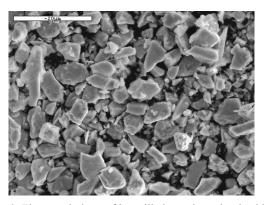
**Fig.3.** The morphology of jet-milled powder pulverized by the initial fresh strip casting at classifier speed of 7000 rpm.
