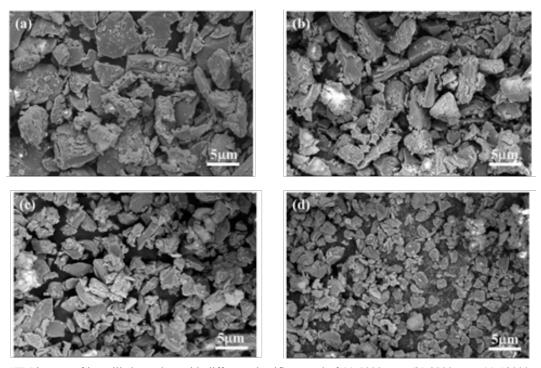
**Fig.1.** SEM images of jet-milled powders with different classifier speed of (a) 7000 rpm, (b) 9000 rpm, (c) 12000 rpm, (d) 20000 rpm.
