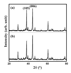
**Fig.5.** The XRD patterns of the surface perpendicular to the alignment direction of the (a) "initial sintered block" and (b) "reproduced sintered block".
