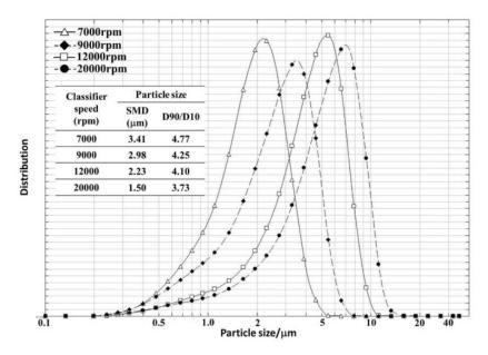
Fig.2. Particle size and distribution of jet-milled powders with different classifier speed.
